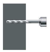
1.Drill three holes in the required position on the wall using a 14mm masonry drill bit, to a depth of 75mm.
